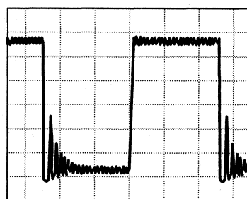
(c) C_L = 310 \text{ pF} , R_L = \text{NO LOAD}
